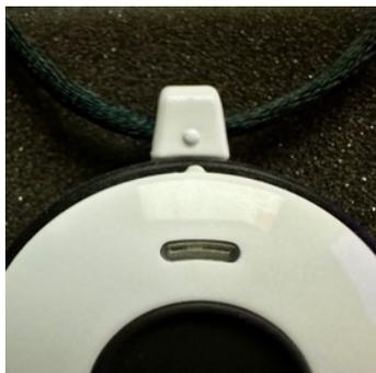
7. Test the pendant making sure the LED is flashing and connectivity was maintained with the FallCall app. (See Section 3: Testing)
