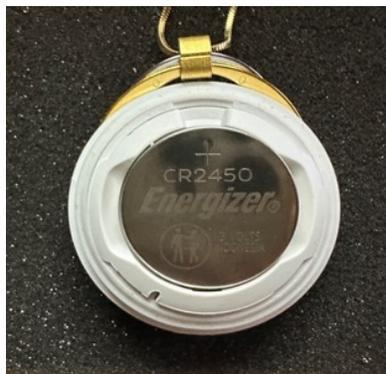
3. Reassemble FallCall Pendant ensuring that the grooves at the top of the inside of the button side are aligned with the slot at the top of the battery insertion side.
